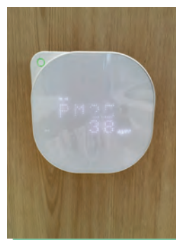
Air quality monitors
